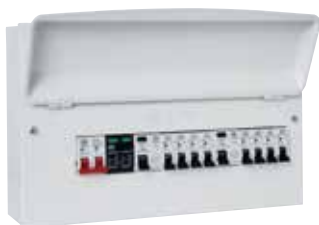
YS8666sMET 16 WAY ENCLOSURE 100A SDC 2 X 100A 30MA RCD 8 X MCBs (2 X 6A, 2 X 16A, 3 X 32A, 1 X 40A) 1 X SURGE
